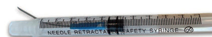
Figure 2. Needle can puncture through the syringe barrel if the plunger is advanced after the safety mechanism has been engaged.
